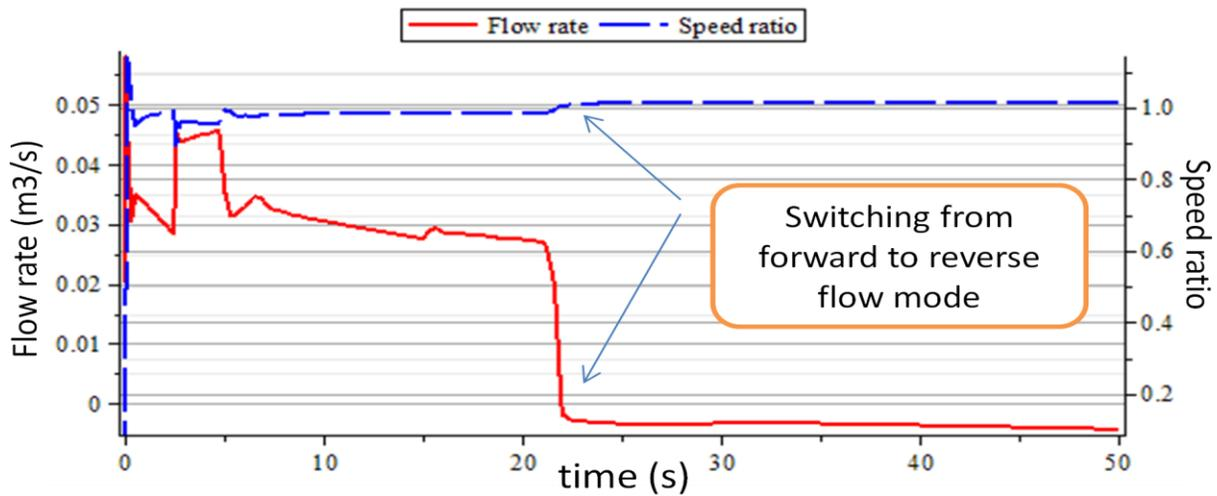
Figure 11: Torque converter flow rate and speed ratio during forward and reverse modes
