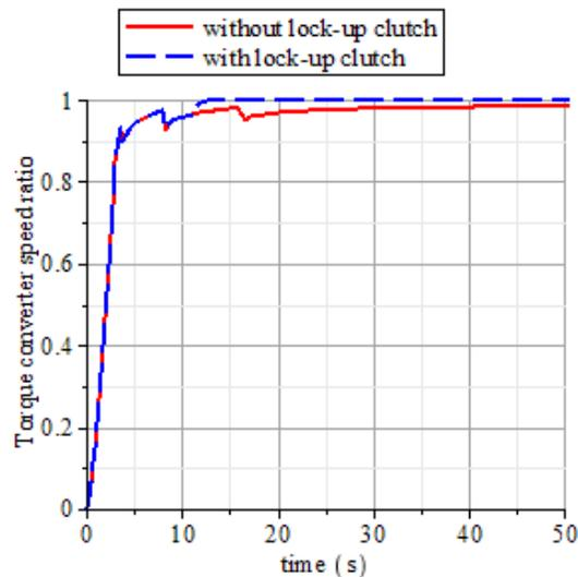
Figure 8: Lock-up clutch effect on speed ratio
