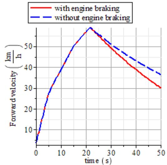
Figure 13: Engine braking effect on forward velocity
