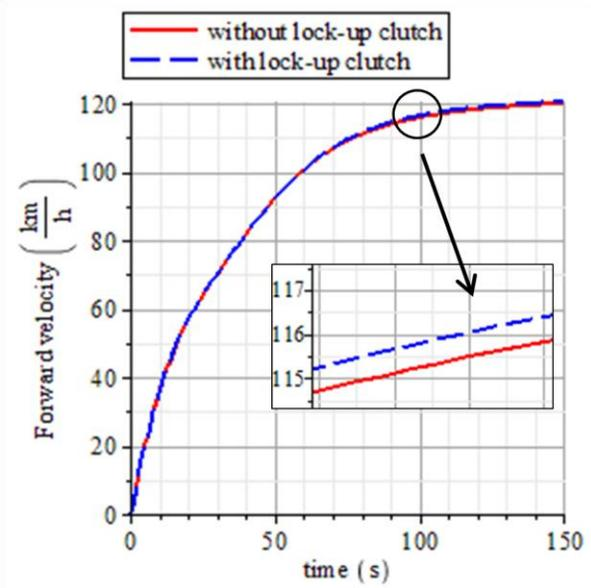
Figure 9: Lock-up clutch effect on forward velocity
