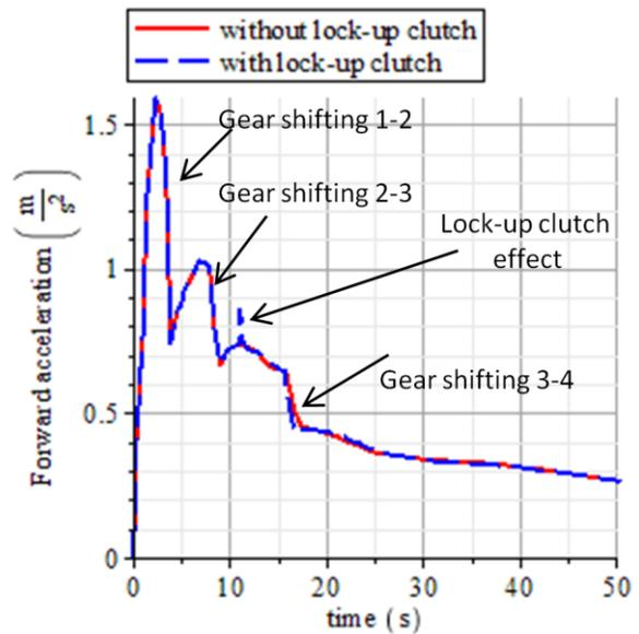
Figure 10: Lock-up clutch effect on forward acceleration
