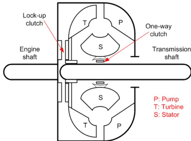
*Figure 2: Cross section of a torque converter*
