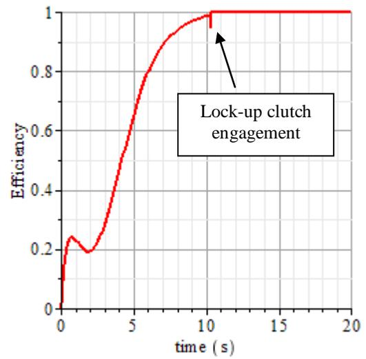
*Figure 5: Efficiency plot (including lock-up clutch effects)*
