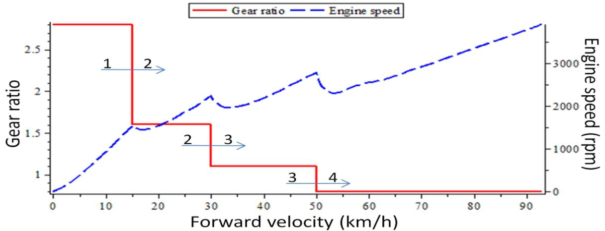
Figure 7: Engine speed and gear ratio variations
