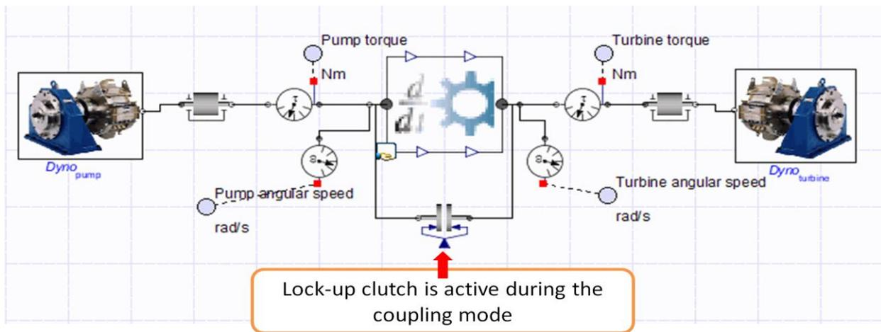
Figure 3: Torque converter test set up in MapleSim
