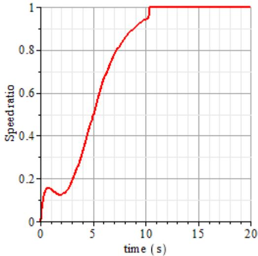
*Figure 4: Speed ratio plot (including lock-up clutch effects)*
