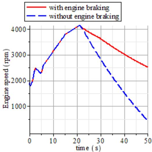
Figure 12: Engine braking effect on rpm
