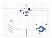
17. Click the input port of the **Torque** component, then drag your pointer to the subsystem boundary and click the boundary once. A real input port is added to your subsystem.
