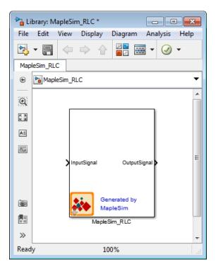
Double-click on the block to open the **Parameter Mask** dialog box that contains the symbolic parameters from the original model (see the following figure).
