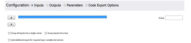
Select **Group all inputs into a single vector** to create a single 'vector' input port for all of the input signals instead of individual ports. The order of the inputs are the same as given in the S-function mask window.
