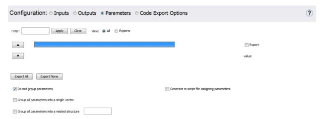
Select **Group all parameters into a single vector** to create a single parameter 'vector' for all of the parameters in the S-function. If not selected, the S-function mask will contain one parameter input box for each of the S-function parameters.
