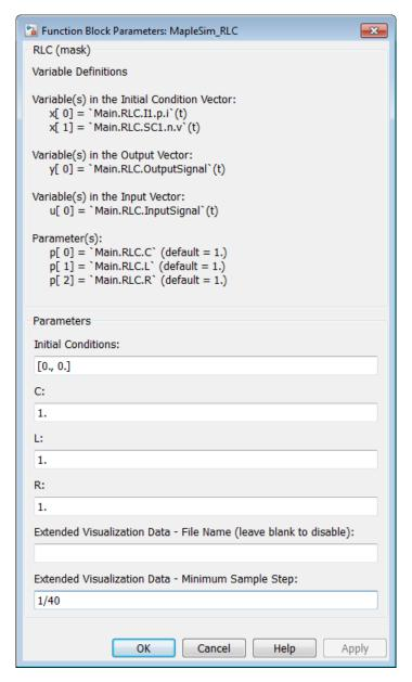
You can set parameters for the block from this mask. For 2016.2 and later versions of the MapleSim Connector, the two *Extended Visualization Data* parameters are used to create data files that can be imported back into MapleSim. This lets you see view the results from executing the block in MapleSim (see the following section, **Enabling Extended Visualization Data**, for details).
