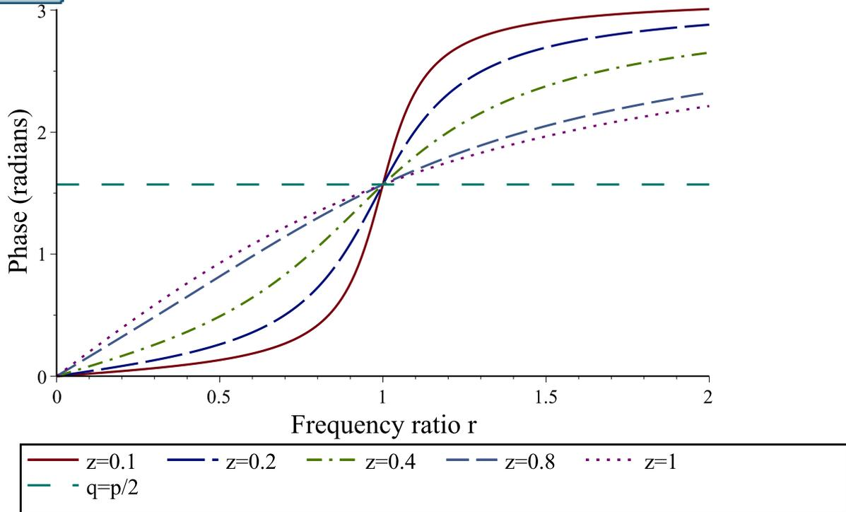
This plot shows that as the driving frequency increases, the phase difference between the steady-state response and the driving force increases from 0 to  $\pi$  and is equal to  $\pi/2$  ( $90^\circ$ ) at the natural frequency of the system.
