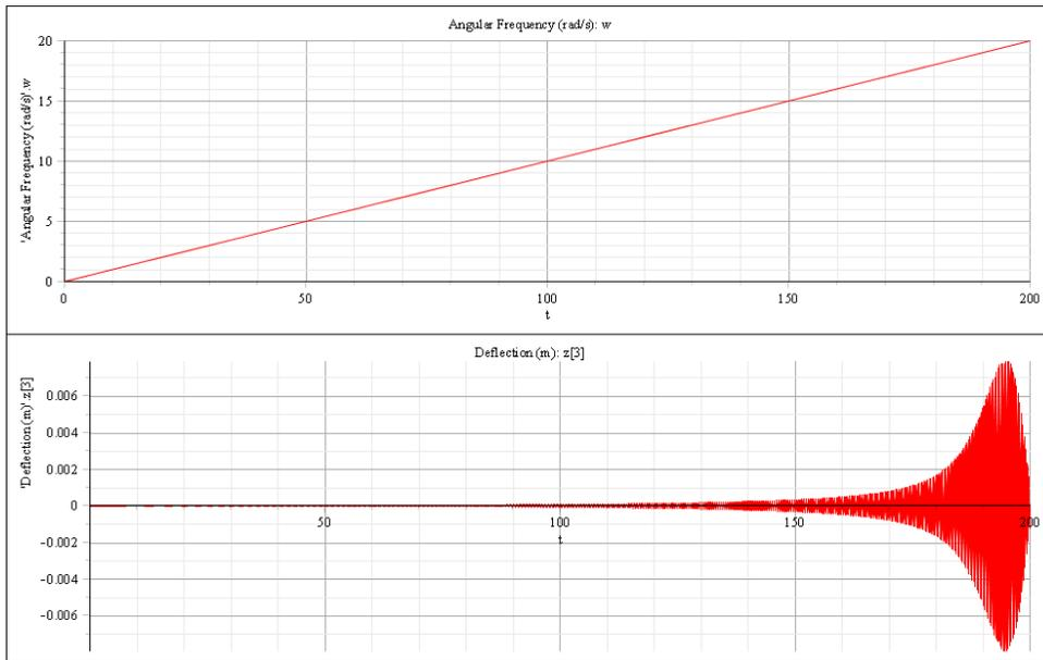
**Fig. 11: Angular frequency (rad/s) and tip deflection (m) vs. time  $t$  (sec) plots for  $h=5$  m.**
