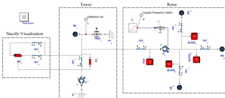
**Fig. 7: Wind turbine simulation component diagram**
