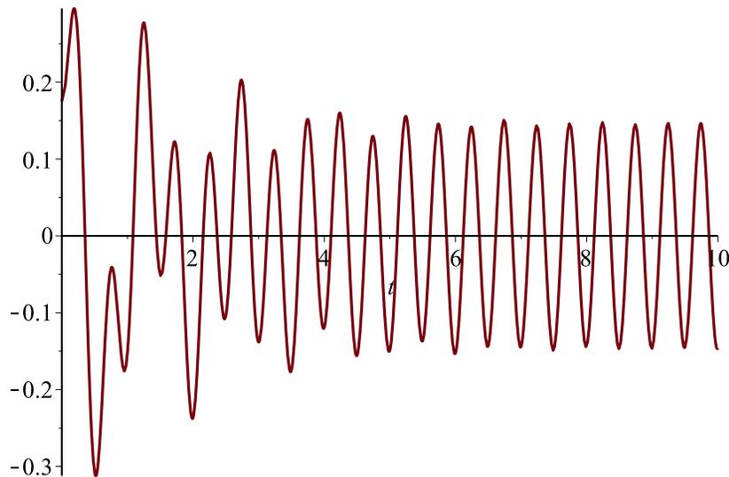
From this plot, it can be concluded that the maximum displacement is approximately 0.29 rad at approximately 0.17 seconds.
