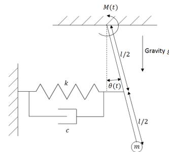
Fig. 3: Spring-pendulum example
