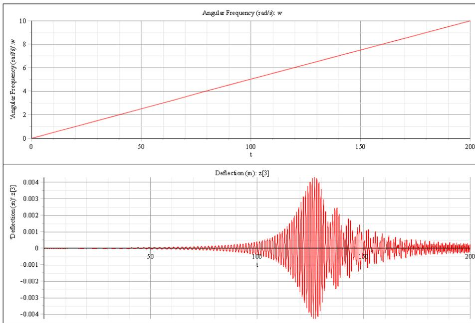
**Fig. 10: Angular frequency (rad/s) and tip deflection (m) vs. time t (sec) plots for h=10 m.**
