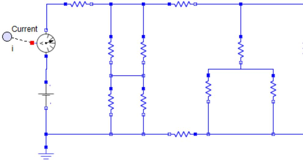
The configuration of circuit elements clearly affects the behaviour of a circuit. Resistors connected in series or in parallel are very common in a circuit and act as a voltage or current divider. We use Kirchhoff's laws to understand the extent of these configurations and to analyze resistive circuits. These principles also help introduce 'equivalent' circuits, exploring ways to simplify a circuit for easier analysis.
