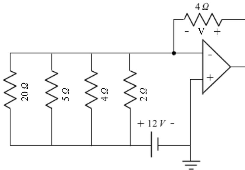
Figure 11: Summing amplifier circuit diagram
