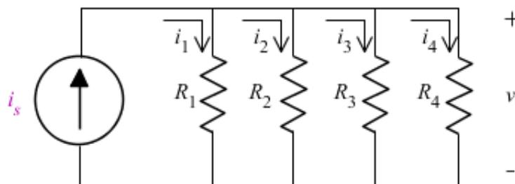
Figure 4: Parallel circuit of resistors
