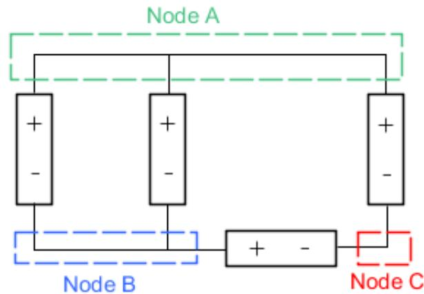
Figure 1: Nodes in a circuit with arbitrary elements
