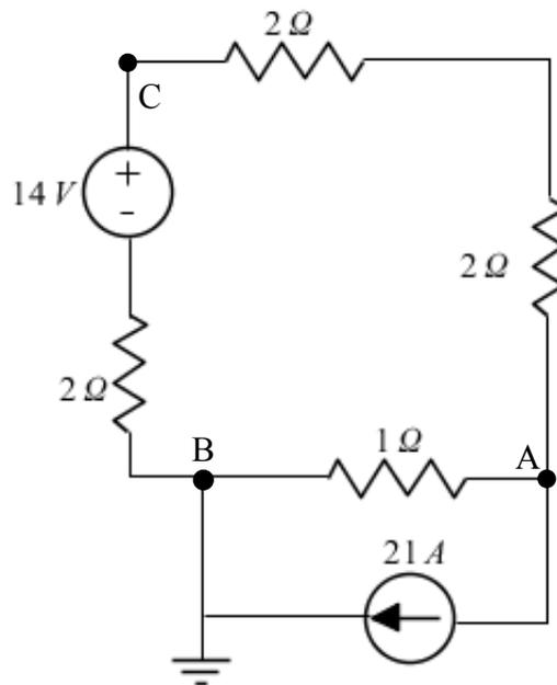
Figure 7: Equivalent circuit - Combining series and parallel circuits
