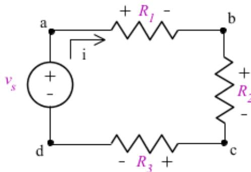
Figure 2: Circuit of resistors in series
