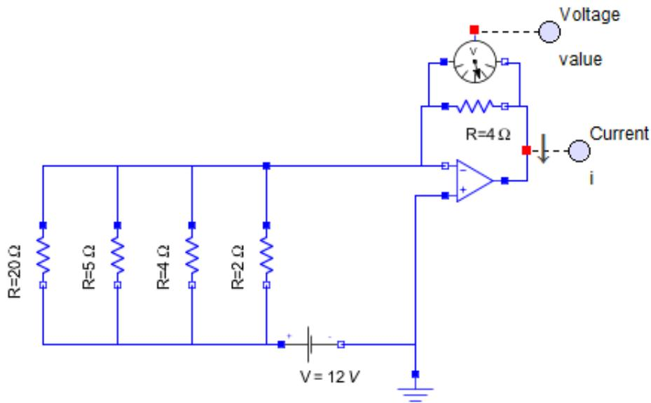
Figure 12: MapleSim diagram of a summing amplifier
