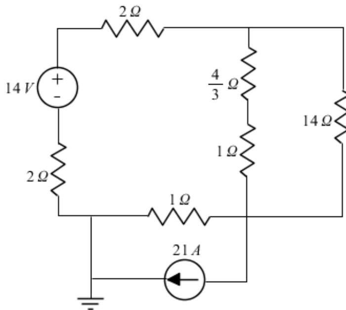
Figure 6: Equivalent circuit - Combined parallel resistors
