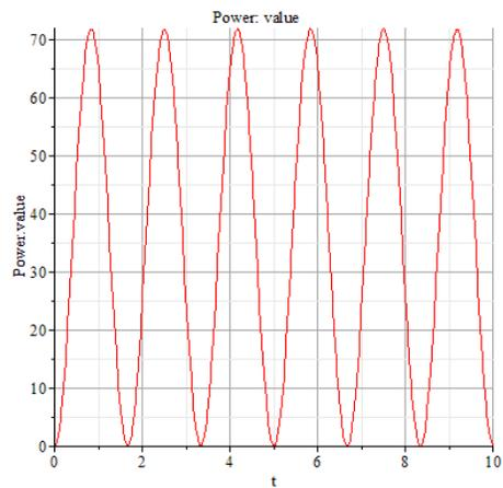
Figure 1.2: Power of a resistive circuit
