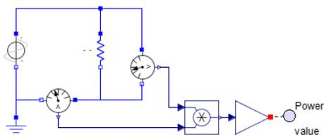
Figure 1.1: Simple R circuit with ammeter and voltmeter
