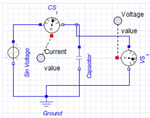
Figure 3.1: A sin signal attached to a capacitor with ammeter and voltmeter connected.
