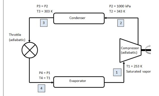
Additionally, a P-h-T chart with the refrigeration cycle will be plotted.
