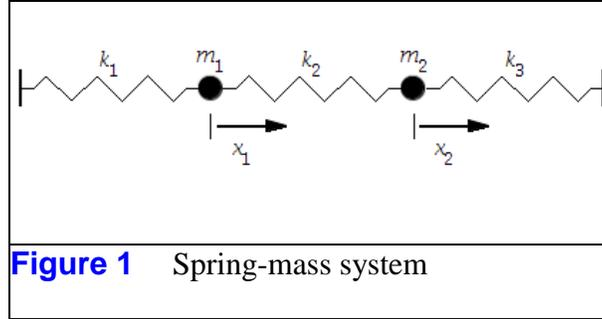
These equations can be cast into the form  $M\mathbf{x}'' + K\mathbf{x} = \mathbf{0}$ , provided the following definitions are made.
