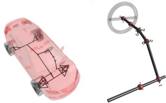
Fig. 2: The developed vehicle model in MapleSim
